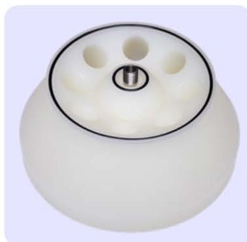
C-R-FA5308 rotor without included sealed lid.
